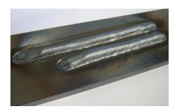
The HD -High Deposit- process, available both in short (standard) and pulsed (optional), allows to execute weldments at very high speed to offer higher and higher yields of the welding plants.
