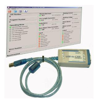
**Kit Robot Analyzer** (art.125.01): when the **real-time monitoring of the communication** between the welding power source and the CNC/Robot Controller is necessary, during either the integration of the welding system or its normal operation, Cebora offers a "sniffer" which lets you to achieve that in an extremely intuitive and complete way.
