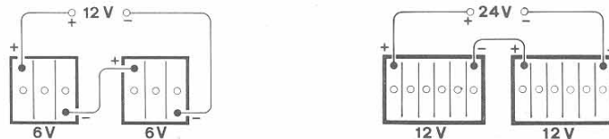
Fig. 2 - CONNECTIONS TO BE USED ONLY IF NECESSARY
