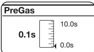
The adjustment can vary from 0 to 10 seconds.
