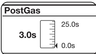
The adjustment can vary from 0 to 25 seconds. To access this function, simply highlight it using the knob **B** and press it for less than 2 seconds. The display screen **A** shows the adjustment bar. The figure can be changed and confirmed by pressing the knob **B** for less than 2 seconds.
