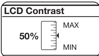
The adjustment may range from 0 to 100%. This function can be used to increase or decrease the brightness of display screen **A**.
