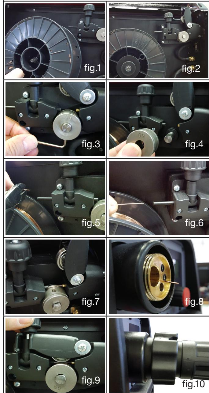
**NOTE.** During the fitting sequence, the welding machine must be switched off to prevent the moving motor roller representing a risk for the operator.
