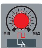
During **MMA** welding, it adjusts the percentage of “arc-force” (N) current; essentially it adjusts a current that produces the electrode transfer.
