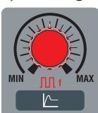
During **MMA** welding it adjusts the “hot-start” current time (L), expressed in hundredths of a second; essentially, it sets an overcurrent that serves to improve striking. It does not make any adjustment during **continuous TIG** welding.
