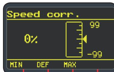
Rotate by one step knob **M1**: display **D3** will show the page corresponding to the wire speed correction.
