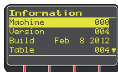
When the welding machine starts, the display **D3** shows for about 5s, a few information about machine status (see par. 7.4 Information menu) including the firmware version.
