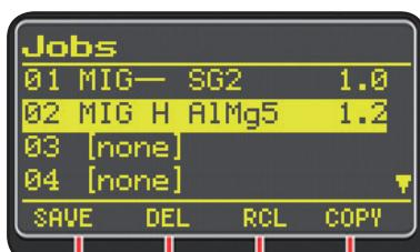
The "Job" program number, the welding process and the wire diameter are shown on the display.
