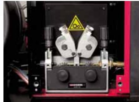
**SOUND MIG 3840/T STAR PULSE** (art. 387) è un **inverter three-phase power source with pulsed** synergic operation, intended for professional use, wherever top-quality welding is required along with high productivity. It is also a multi-process power source, able to weld in MIG-MAG, TIG (contact ignition with "LIFT" system by Cebora) and MMA mode. It is supplied with **integrated torch cooling unit and 4 roller (ø 40 mm) wire feed unit**.
